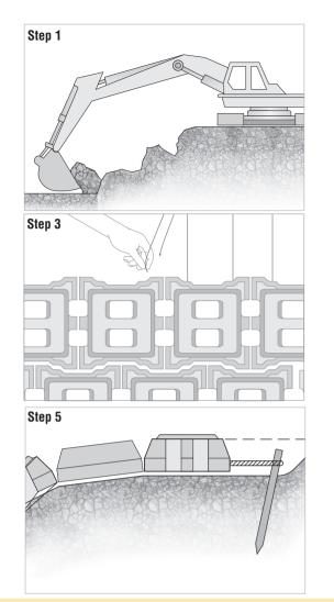
Step 1: Site preparation, excavation, trimming & compaction Prior to laying Armorflex, the base material must be profiled to line and level and should be compacted to a firm and even finish. Obstructions, such as roots and projecting stones should be removed as the quality of the preparation will be reflected in the finished surface. The angle of repose of the in situ material must not be exceeded. Maximum desired slope is 1:1,5
