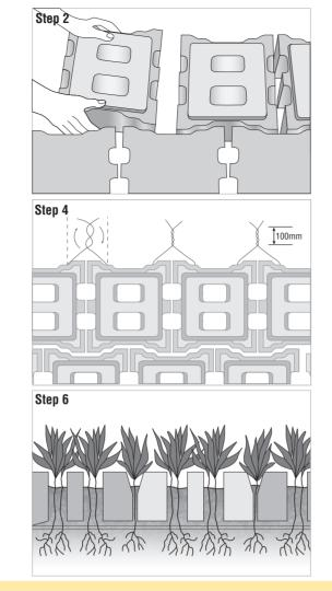
a 5 mm diameter polyester rope can be used. In certain situations wiring up may not be necessary. Generally the wire will be threaded perperdicular to the flow.
