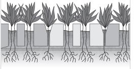
Step 1: Site preparation, excavation, trimming & compaction Prior to laying Armorflex, the base material must be profiled to line and level and should be compacted to a firm and even finish. Obstructions, such as roots and projecting stones should be removed as the quality of the preparation will be reflected in the finished surface. The angle of repose of the in situ material must not be exceeded. Maximum desired slope is 1:1,5
