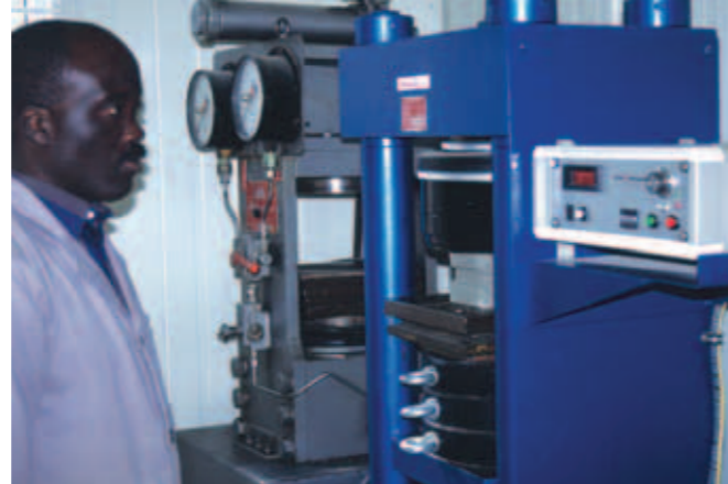
Technicrete Composite Pack element under proof compression test.
