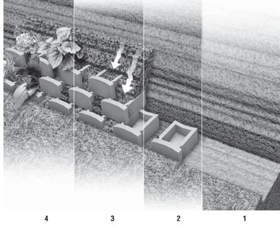
Earthform garden blocks can be stacked up to eight layers high provided that the ground is suitable and that no additional loads are applied at the top of the embankment. For a higher wall an engineer's advice should be sought to comply with Municipal bylaws.
