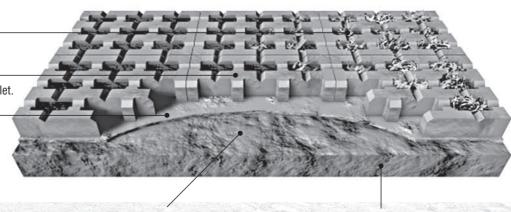
Surface of layer works to standard specifications SABS 1200 MJ. (max. 10mm in 3m)
