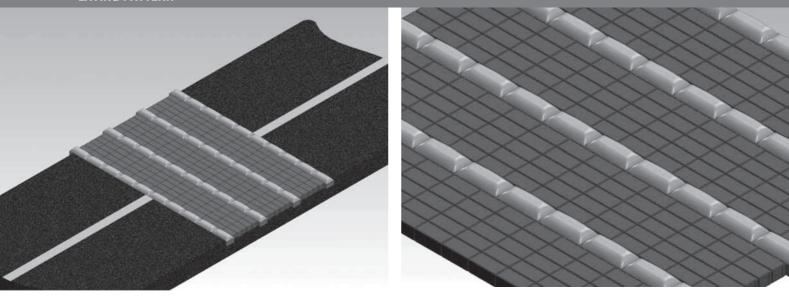
Ripplesett Blocks must be spaced 450mm-550mm apart to create the 'Drag' on a vehicle to reduce speeding. Motorists must be advised of this obstruction before they drive over this calming system.
