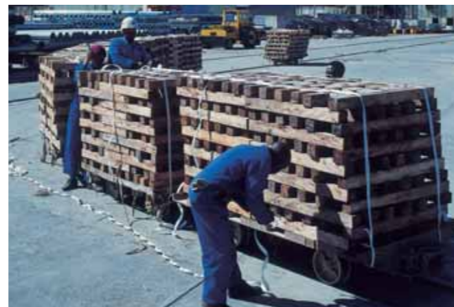
Manufacture carried out on shaft bank where the composite units are packed directly onto mine cars reducing transport and handling costs.
