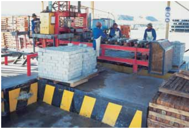
Manufacture carried out on shaft bank where the composite units are packed directly onto mine cars reducing transport and handling costs.
