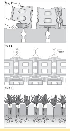
a 5 mm diameter polyester rope can be used. In certain situations wiring up may not be necessary. Generally the wire will be threaded perpendicular to the flow.
