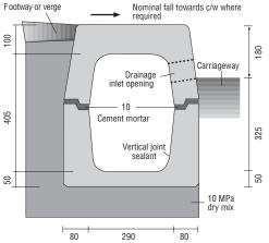
protected to prevent backing concrete entering the Beany Block System. (Unless tops without drainage openings are specifically ordered).
