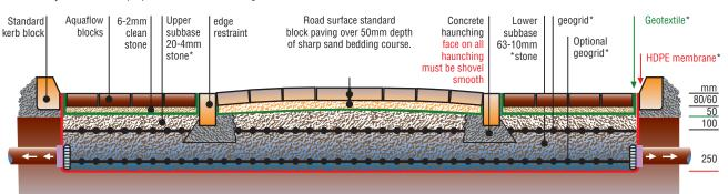
\* Hydraway fin drain connected to 110mm PVC-U pipe with Technicrete top hat seal
