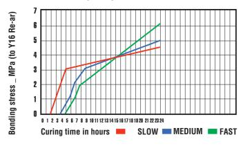
HT33 Binder and grout blends This is a unique cementious product with extraordinary flow properties and long term strength gain. The HT33 can be supplied as a premixed pumpcrete ideal for pumping as a structural mix into difficult areas such as Box Fronts, or as a fine grout for consolidation of loose material. The HT33 is easily converted
