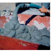
into a foam product suitable for mixing into a tailings mix for stope support as a yielding grout pack.
